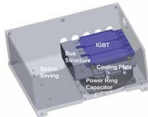
Figure 2 shows the “stacked” inverter design after the integration of the ring capacitor and the laminar bus plate. By now combining both aspects of vertical integration and the low temperature rise characteristics of the capacitors, an increase to 50% or more volume reduction is realistically possible. These improvements clearly translate into weight and cost reductions.
