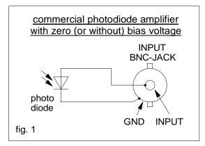
Some amplifiers only have a fixed bias voltage or the bias cannot be trimmed to near zero. In this case it is required to draw the ground level (which is not available on the input jack) from other sources, e.g. the output jack, special connectors or even from the housing. Please refer to the amplifier's manual and figure 2.
