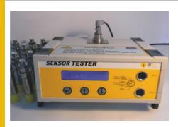
The **Sensor Tester** is used for UV sensor calibration.
