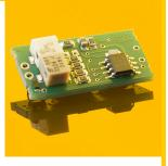
Other modules with medium gain (AMPCON\_MED, up to 2,5 $\mu$ A) and low gain (AMPCON\_LO, up to 250 $\mu$ A) are available. Alternatively, please refer to the below instruction for changing the gain.
