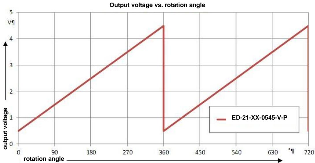
figure 3: Output voltage vs. rotation angle
