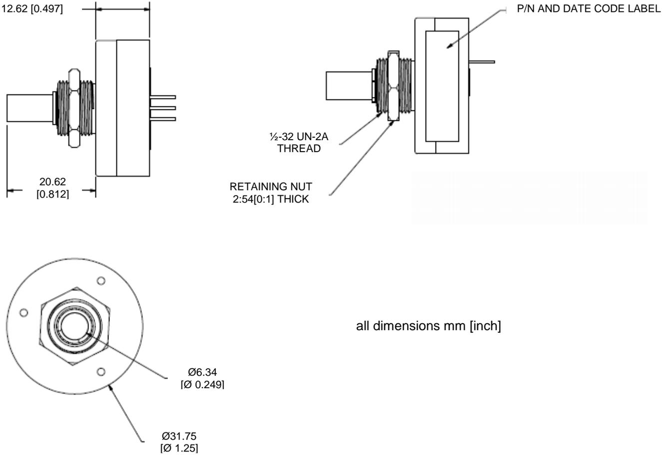
figure 1: Dimensions of the ED-21
