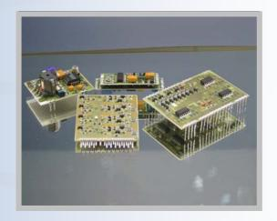
Hybrid circuits are subjected to both passive and active trimming by modern laser techniques, thereby offering closer working tolerances.
