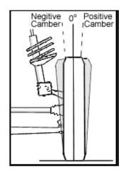
Camber is the angle of the wheel, measured in degrees, when viewed from the front of the vehicle.
