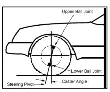
Caster is the angle of the steering pivot, measured in degrees, when viewed from the side
