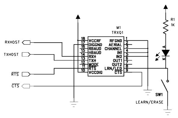
In some addressed mode applications the learn/erase components may not be required and the LRN/LED pin could be connected to the host micro controller which would be programmed to handle the functions of this pin.
