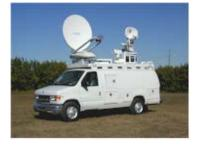
are known as antenna positioner/controllers. These are electronic devices, which use various sensors to measure, then automatically adjust the antenna to the proper azimuth (deviation from true north) and elevation (slope angle) positions required.
