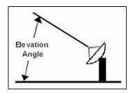
The elevation angle is normally measured using an electronic inclinometer, with a minimum measurement range of 0-90 (+/-45)
