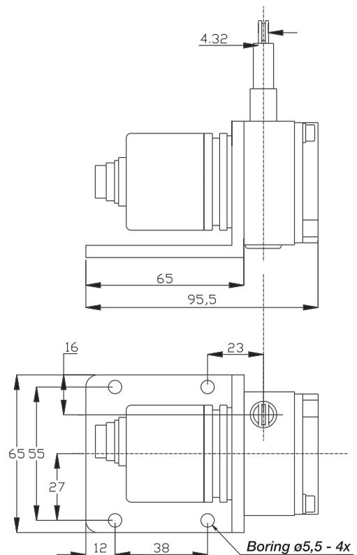
All details in mm and dependent on the encoder configuration
