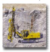
construction industries. They are primarily employed for surface drilling and/or ëdrill and blastí tunneling tasks, usually through solid rock. Working under a Geologists direction, these rig operators drill blast holes up to 100 feet deep, at precise
