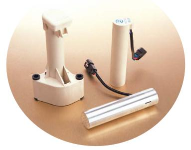
element whose buoyancy causes slight relative motion. This small movement of the magnet-topped float, in relationship to a Hall Effect device, provides a definitive indication of fluid level with exceptional repeatability.
