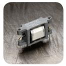
A fully screened relay offering low RF loss and high current carrying capacity, which was developed with RF design engineers in the radio communications industry. The relay coil is totally enclosed in a copper screen, resulting in lower self-heating and RF loss, and Rhodium contacts are used in the vacuum reed switches, yielding higher carry currents for a given frequency and ambient temperature.
