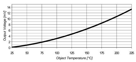
Conditions: Distance Thermopile/Black Body 5 cm, emissivity= 1, surrounding temperature 25°C
