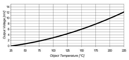
Conditions: Distance Thermopile/Black Body 5 cm, emissivity= 1, surrounding temperature 25°C
