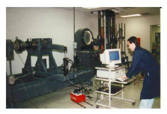
Force calibrations to: 300,000 lbs. Torque calibrations to: 250,000 in-lbs
