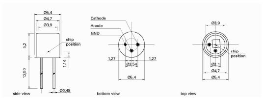
Selection code "18ISO90" → TO18 Ni plated housing, 5.6 mm diameter, 5.2 mm height three gold plated pins (Anode and Cathode isolated, additional third pin for optional grounding of the body).
