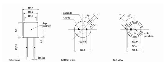
Selection code "18" → TO18 Ni plated housing, 5.6 mm diameter, 5.2 mm height two gold plated pins (Anode grounded and Cathode isolated).
