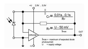
The adjacent design gives an example of a simple amplifier circuit. At the left side the photodiode is shown. The upper connection is the Cathode (isolated pin of the photodiode) and the lower connection is the Anode (usually grounded pin of the photodiode).
