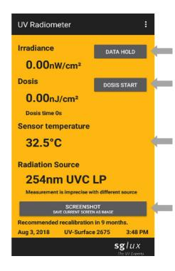
Drop-down menu The radiation source (calibration) can be selected here. The advanced view is also selectable.
