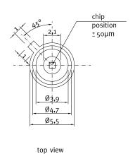
UVB-only SiC based UV photodiode A = 0,50 mm<sup>2</sup>
