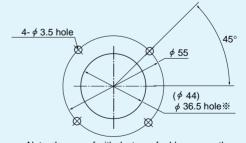
Note: In case of with dust proof rubber cover, the dimensions of " $\mbox{\ensuremath{\%}}$ " part changes to  $\phi$  44 mm. hole.
